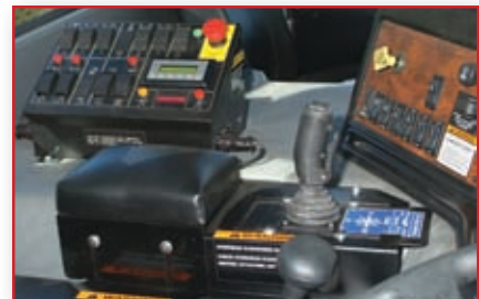
PLC logic controller with performance data capture and service minders
