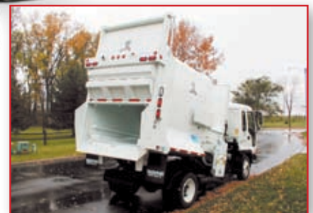
Satellite model with tilt-for-transfer body
